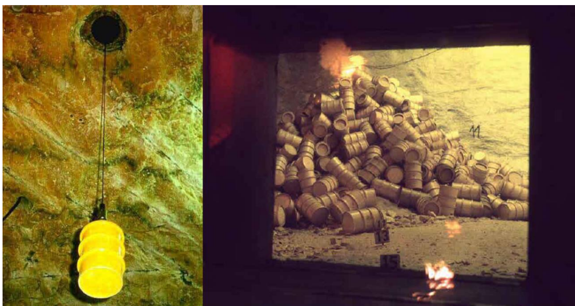
Fig. 8: Left: Lowering of a waste drum into the emplacement chamber for Intermediate Level Waste. Right: Emplacement chamber for Intermediate Level Waste [15].
