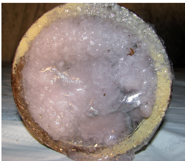
Fig. 11: Rock salt particles consolidated by a sodium silicate solution. The inner diameter of the tube is 100 mm.
