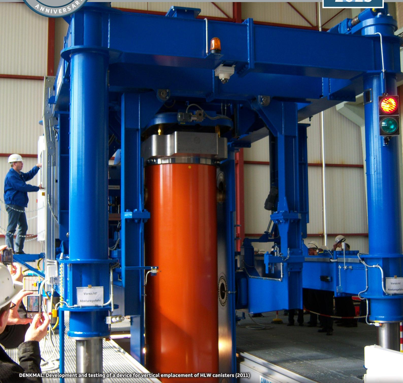
DENKMAL: Development and testing of a device for vertical emplacement of HLW canisters (2011)
