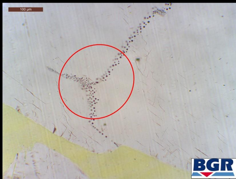
Fluid inclusions in crushed salt raw material
