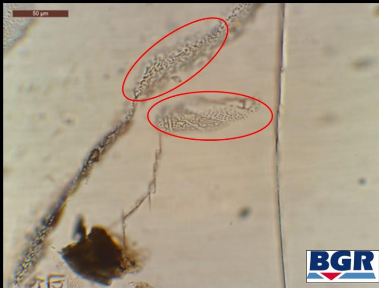
Fluid inclusions (oedometric compaction; 50°C, max. 30 MPa)
