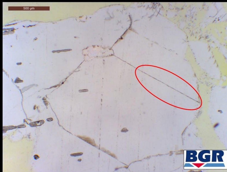
Microcracks in crushed salt raw material
