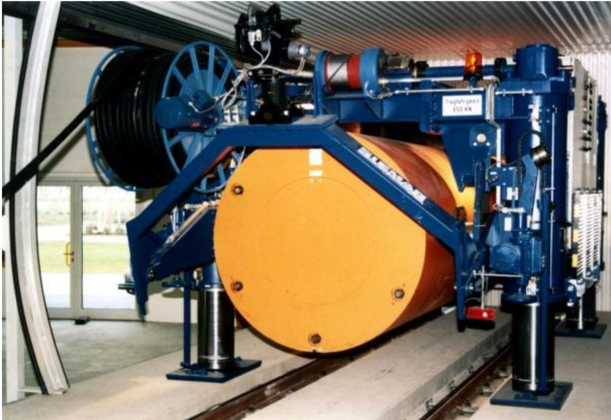
**Figure 5.19: Emplacement device for the drift disposal of POLLUX® casks**
