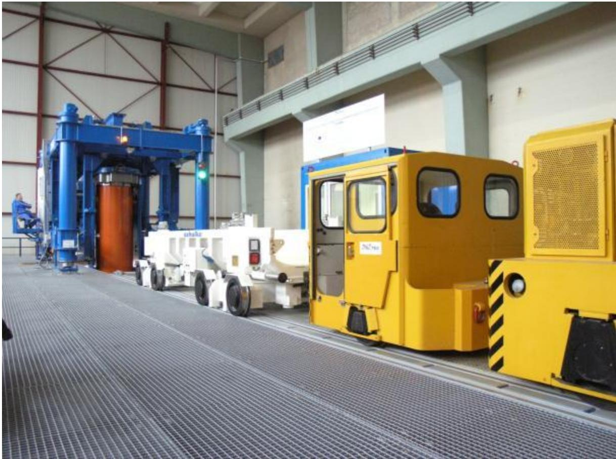
**Figure 5.20:** Test stand for borehole disposal of canisters [Filbert et al. 2010]
