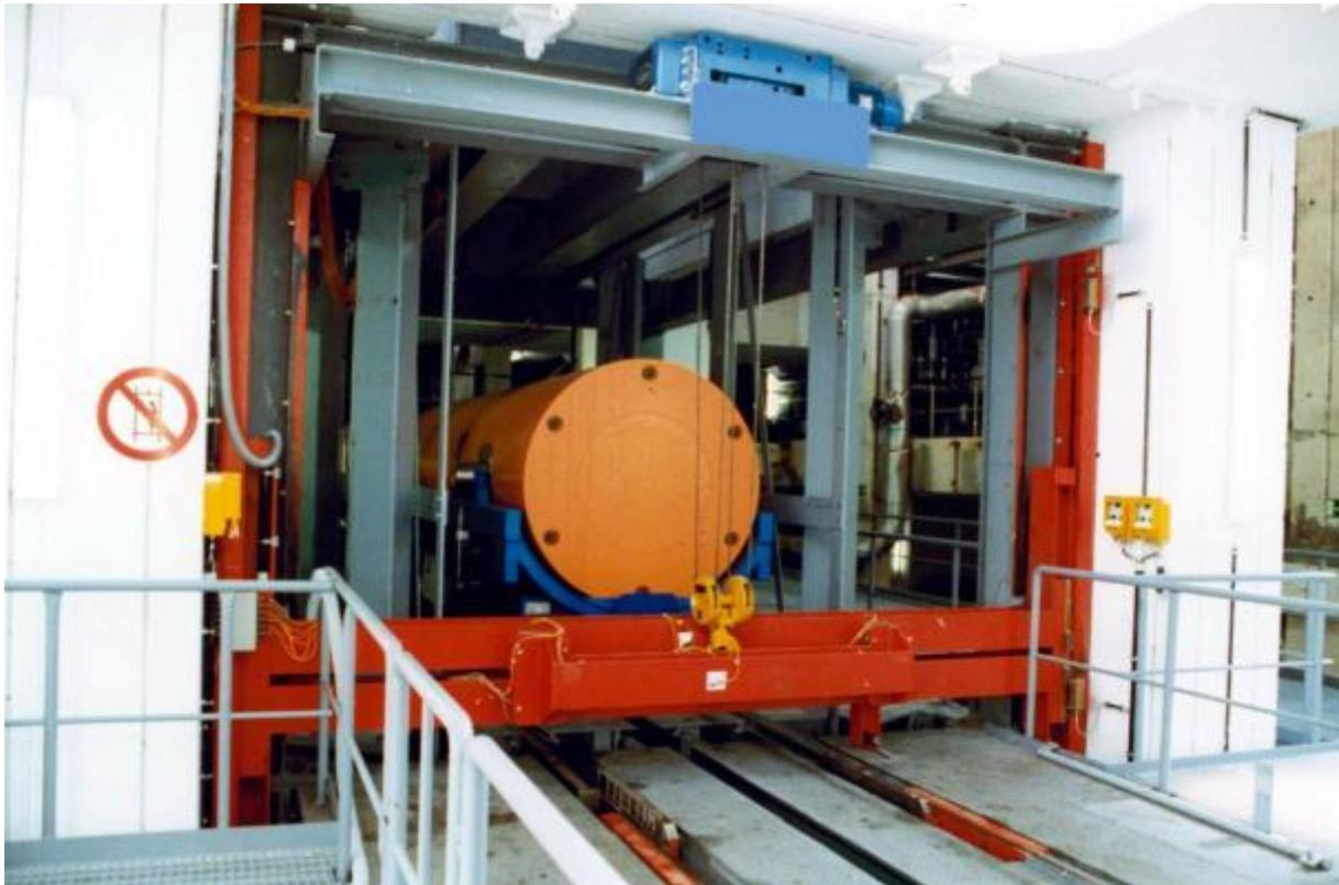
**Figure 5.18: POLLUX® casks on transport cart in the hoisting cage**
